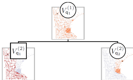
Fig.: Illustration of a binary wedge split based on two nodes q_1 and q_2 .
